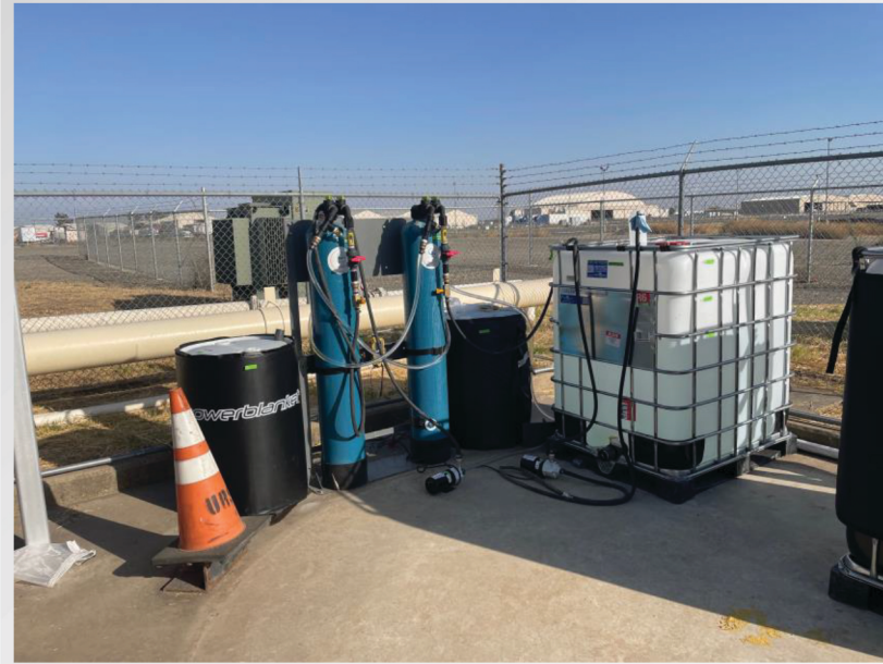
DEXSORB provided 5,000x of PFAS concentration factor in this field demonstration
