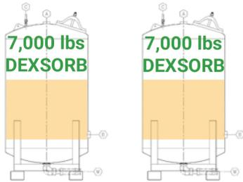
DEXSORB packed bed filtration (two 7,000-lb vessels) for removal of **PFOS and 6:2 FTS**; **Replace 7,000 lbs DEXSORB every 36 weeks**
