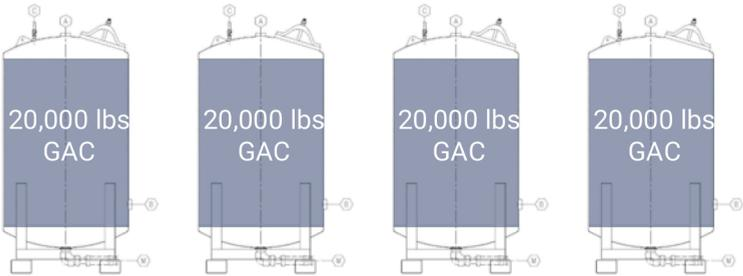
GAC packed bed filtration (four 20,000-lb vessels) for removal of **PFOS and 6:2 FTS**; **Replace 20,000 lbs GAC every 6 weeks**
